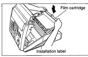
Make sure that the blue label on the cartridge matches the one on the unit.
