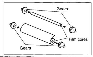
6 Insert the blue gear into the blue core of the new film.
