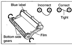
Install the film cartridge into the unit.
