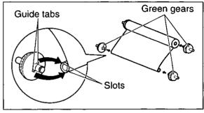
8 Insert the film into the cartridge so that the blue gear matches the blue label on the cartridge.
