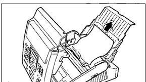
If the film is slack, tighten it by winding the bottom side gears.
