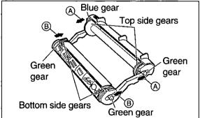
Remove the four gears from the used film cores.
